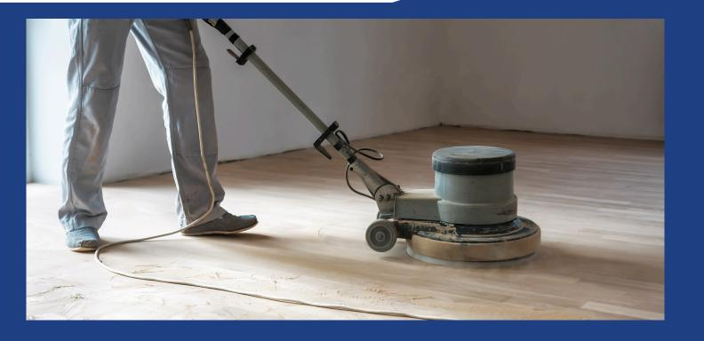
Used for: Sanding wooden floors smooth for finishing.
