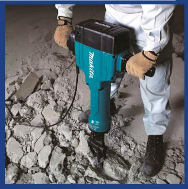
**Used for:** Breaking concrete, old paving, bricks, and asphalt.
