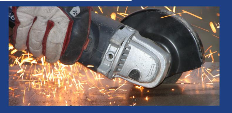
**Used for:** Cutting, grinding and polishing metal, stone or tile.
