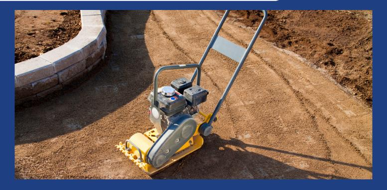
**Used for:** Flattening and compressing soil, sand, gravel and sub-base before laying patios or driveways.
