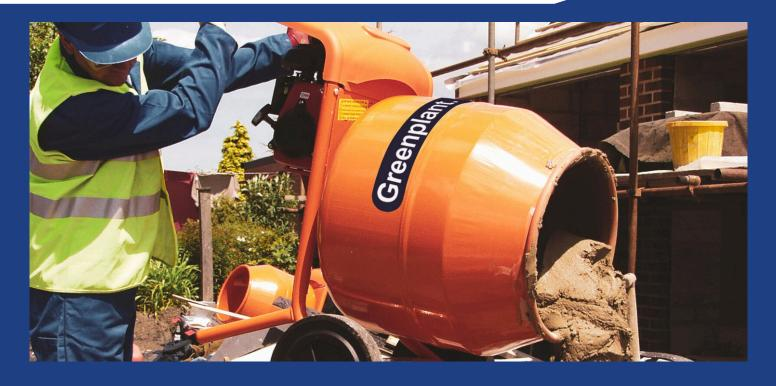
**Used for:** Mixing sand, cement and water for mortar or concrete jobs
